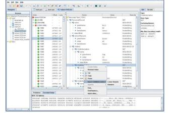
To decode values just choose the ASN.1 syntax and the encoding rules that you want to use. The decoded values are then displayed in the main panel using a tree representation. Errors during decoding are skipped.
